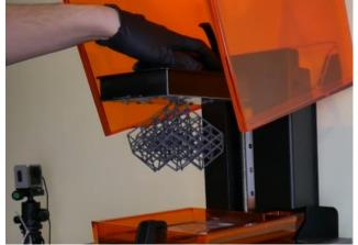
2. Place the buid platform directly from the printer to the Form Wash
