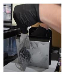
**4.** Cut the supports and allow your print to fully dry before placing it in the Form Cure.
